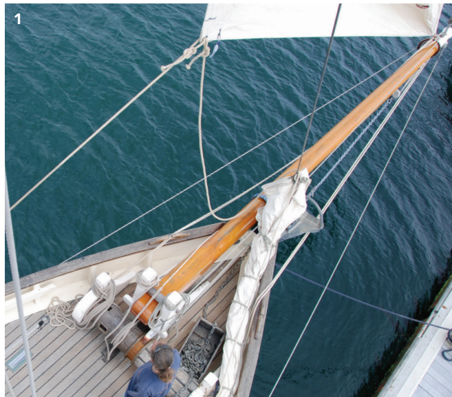
Bringing the jib in. 1: Post crew on the foredeck to haul in the traveller from the end of the bowsprit. 2: Flake the halyard so that it will run free through the masthead block. 3 and 4: Helm bears away to take the drive out of the jib and the traveller is hauled back to the bows. 5: The halyard is let out under control and the foredeck crew haul in the sail... smartish.
