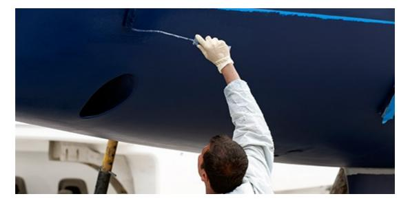
Apply the paint evenly onto the hull avoiding overloading the roller, the more time and care taken to apply the antifouling the better its longevity and performance, too often antifoul failure is blamed on the product rather than the actual cause is poor preparation and application.
